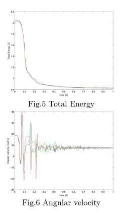
The red, blue and green lines show the result of model 1, model 2, and model 3. The bridge shape of model 1 is rectangular, one of model 2 is trapezoid with long top side, one of model 3 is trapezoid with short top side.
