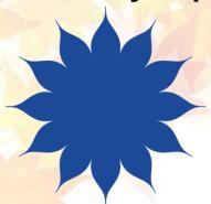
The shape of the currently proposed occulter is a petal shape which suppresses the diffraction of the stellar light as much as possible. Since this shape has a curved outline unsuitable for the deployment structure, the occulter is a very complex deployment style and its cost is expensive.
