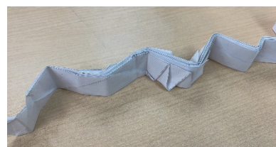
Fig. 13 Folded membrane by bellow folding
