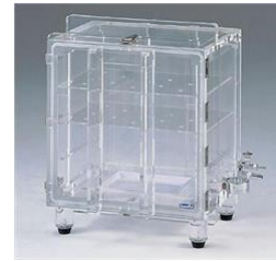
Fig. 4 Small acrylic Vacuum chamber
