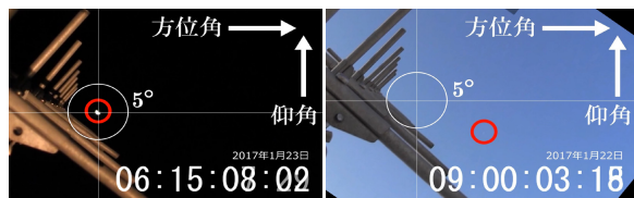
Fig. 10 Antenna angle check by moon tracking①
