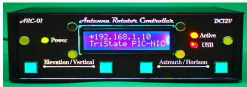
Fig. 5 Flexible controller for antenna rotator “ARC-01”
