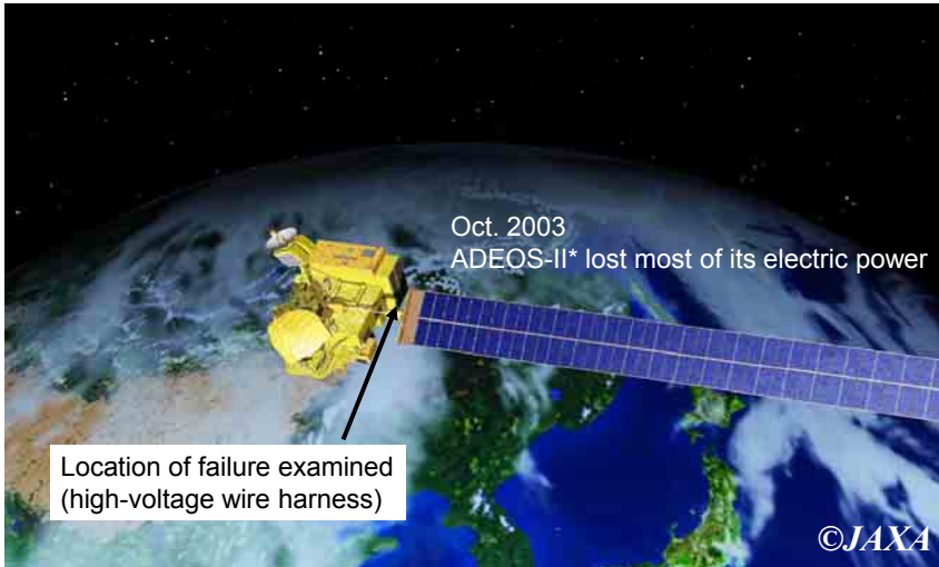
*ADEOS-II: Polar Orbit Satellite: paddle size 3 x 24 (m) (JAPAN)
