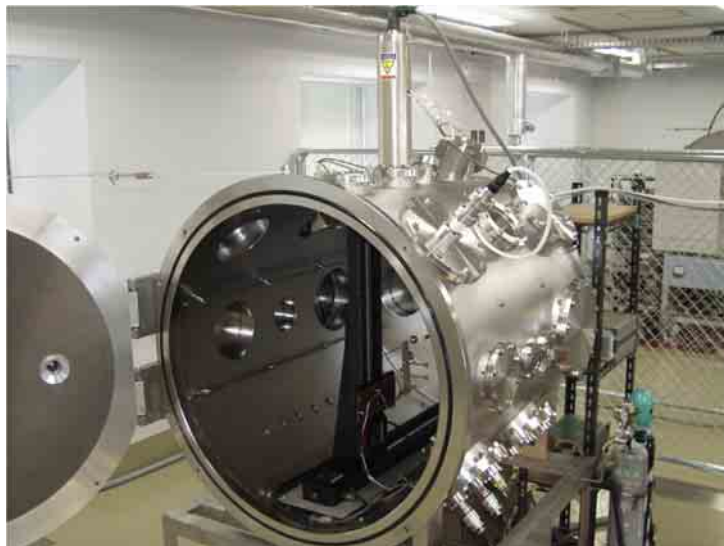
Chamber to simulate Polar Earth Orbit Environment
